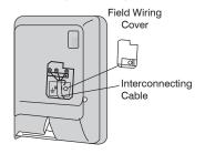
6. Pull interconnecting wire up from back of indoor unit and position in close to the terminal block on indoor unit.
