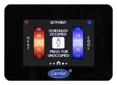
Use this screen to view, adjust, or hold heat and cool setpoints. Use the wheels to adjust setpoints. Drag a wheel up or down or tap the top or bottom of the wheel to increase or decrease by 1 increment.
