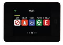
2 Swipe to go to the **FAN** screen and then press and hold the **Fan Button** for 5 seconds to get to the **SYSTEM SETTINGS** screen.
