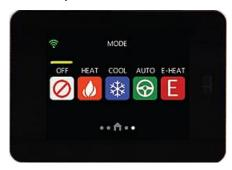
2 Swipe to go to the **FAN** screen and then press and hold the **Fan Button** for 5 seconds to get to the **SYSTEM SETTINGS** screen.
