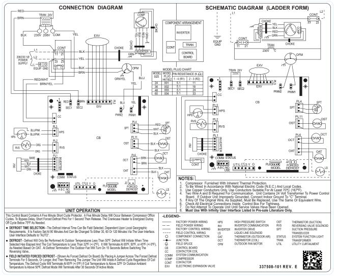
Fig. 1 – Wiring Diagram — Model sizes 2 - 5 tons, 208/230-1
