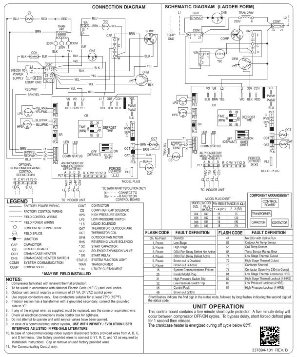
Fig. 1 – Wiring Diagram — Model sizes 2 – 5 tons, 208/230-1
