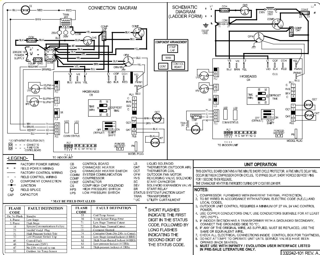
Fig. 1 – Wiring Diagram — Model size 24, 208/230-1
