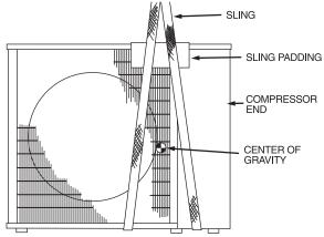
Fig. 2 — Lifting Unit with Sling
