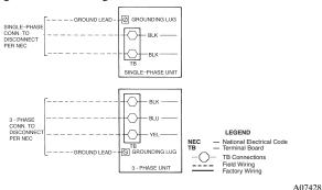
Fig. 4 — Line Power Connections
