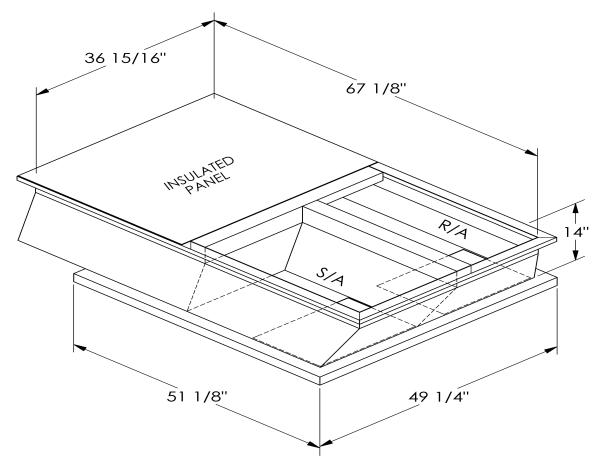
ONE PIECE WELDED CONSTRUCTION
