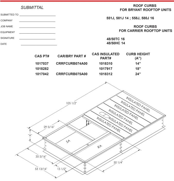
MITERED TOP CORNERS ROOF CURB IS FABRICATED OF 18GA G90 GALVANIZED STEEL FULL PERIMETER WOOD NAILER PRE-PUNCHED ASSEMBLY HOLES AND HARDWARE INCLUDED FOR DUCT SUPPORT INSTALLATION ROOF CURB IS SHIPPED UNASSEMBLED CURBS ARE INTERNALLY INSULATED WITH 1" THICK 1-1/2 LB DENSITY DUCT LINER
