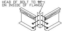
3 BOLT SIDES AND ENDS TOGETHER AS SHOWN USING THE 4 CORNER BRACKETS, BOLTS, AND THE TEK SCREWS PROVIDED.
