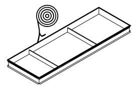
5 REMOVE PAPER BACKING FROM THE PROVIDED GASKETING AND APPLY TO TOP PERIMETER OF ROOF CURB. SET CURB IN PLACE OVER ROOF OPENING, LEVEL CURB AND SECURE TO ROOF.
