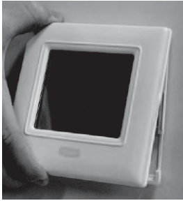
Fig. 11 - Attach Display to Backplate
