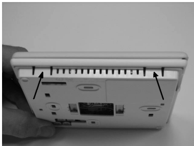
Fig. 5 - Press Tabs to Remove Backplate
