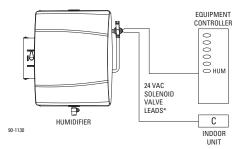
\*Note: Internal float switch circuits are wired in series with one leg of the solenoid
