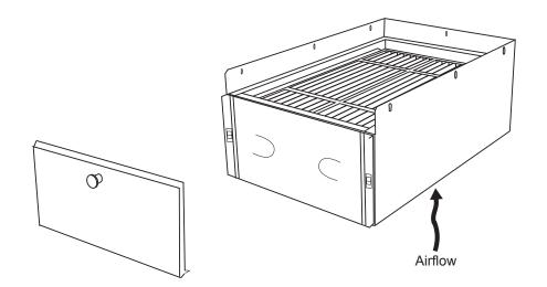
Install FILFNC Media Filter Cartridge in the FNCCAB Media Filter Cabinet.
