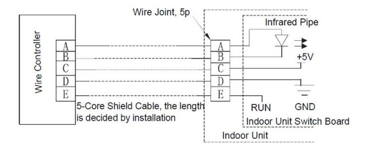
Fig. 2 - Wiring Principle Sketch
