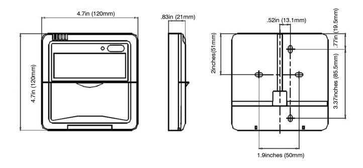
Fig. 1 - Wired remote controller structure size
