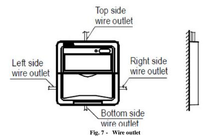
• For exposed mounting there are four outlet positions and three require cutting.
