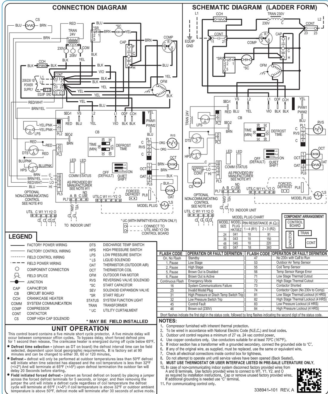
**Fig. 1 – Wiring Diagram — Model size 2 - 5 tons, 208/230-1**
