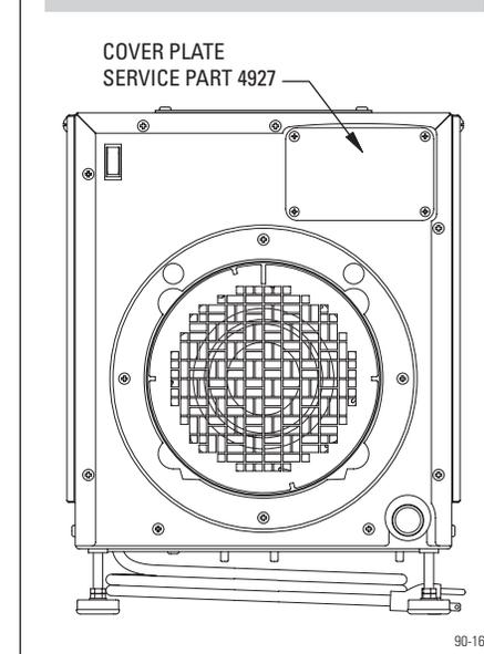
FIGURE 6 – Wiring Access Panel on Outlet
