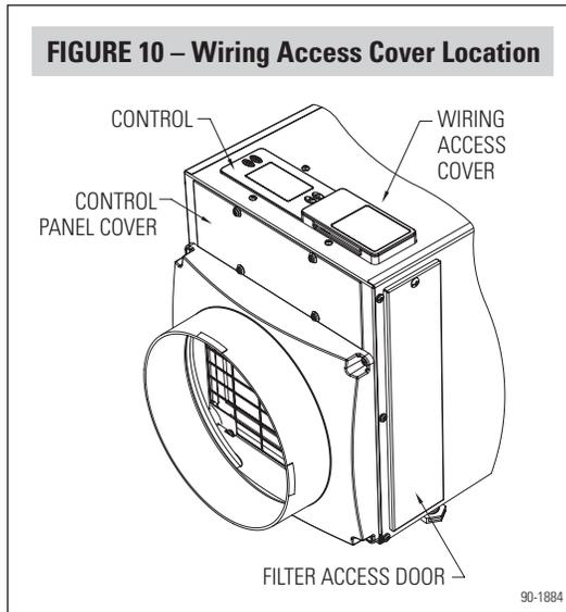
5. Snap the wiring access cover back into place, power up the dehumidifier and use the ON/OFF button to turn the unit OFF (if ON).
