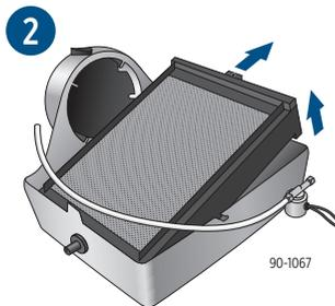
Pull feed tube out of distribution tray, and remove Water Panel® evaporative assembly.
