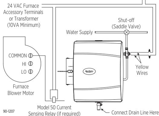
**IMPORTANT:** When Model 50 current sensing relay is used, wire Model 50 current sensing relay into 24 VAC humidifier control circuit only! **Do not install in transformer primary circuit.**
