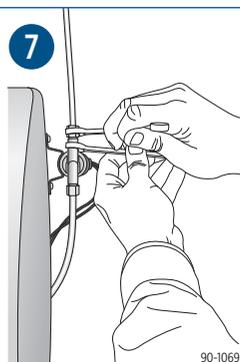
Tighten water line by double wrenching.
