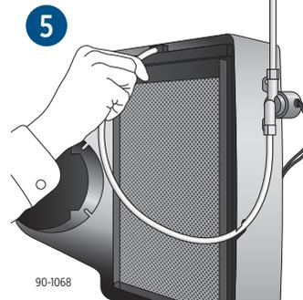
Insert feed tube into distribution tray.
