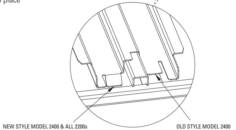
7. For "New Style" Model 2200 and 2400 air cleaners (see illustration at right), press the Styrofoam door liner into the center of the door. For "Old Style" air cleaners, the door liner is not needed.
