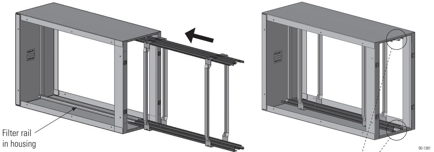
6. Bend the appropriate locking tab to lock the frame into place at the top and bottom.
