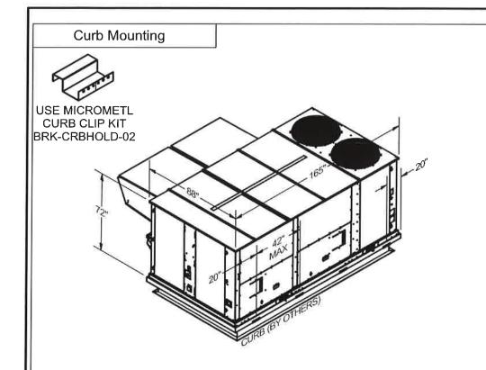
PROVIDE (6) 1/4"-14 x 6" BUILDEX TEK SCREWS AT EACH CLIP PROVIDE (4) CLIPS AT CURB ALONG EA. LONG SIDE OF THE UNIT (8 TOTAL)
