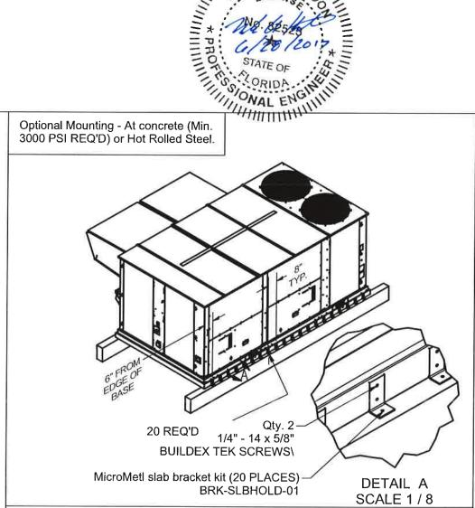
Qty. 1 - 3/8" SAE GR5 Bolt with Nuts and Washers per Clip into Metal Stand (by others), or 3/8" Dia. HILTI KWIK-BOLT TZ Expansion Anchor with 2-1/2" minimum embedment, 2-1/2" Edge Distance and space according to amount of clips required. Glen Oaks Ln., WI 53092 -1601 ENGINEERING CROUP, LLC.
